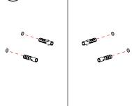
Insert the rawl plugs into the drilled holes.
